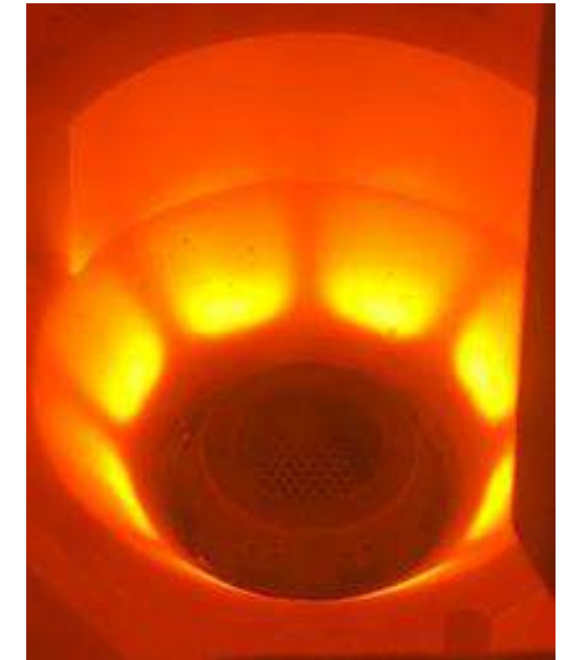
“Proof of Concept” burner 100% Hydrogen
