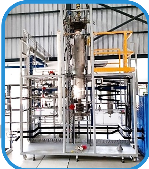
Pilot scale plant of 30 kg CO 2 /day capacity to methanol at JNCASR
